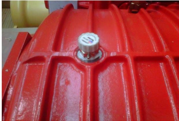
This plug allows the air drainage while first filling and must not be manipulated thereafter: it has to stay at close position.
