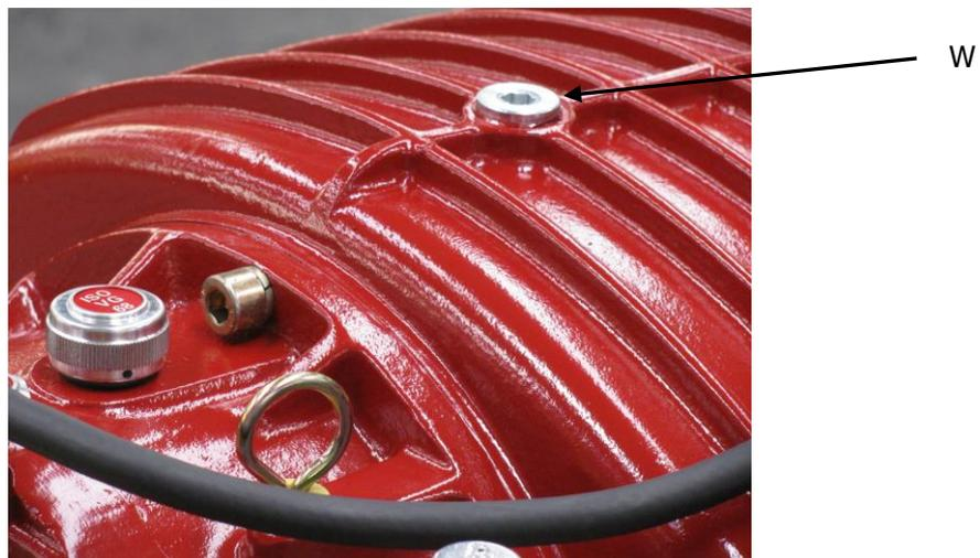
To do that, unscrew the plug W and turn manually the pump rotor to a point where a vane channel comes to the hole which is open now. Take the oil level indicator and measure the depth till the vane edge. Then turn a little bit more the pump rotor and repeat the measure operation till the rotor lateral surface in order to obtain the vanes wearing after both measures subtraction.
